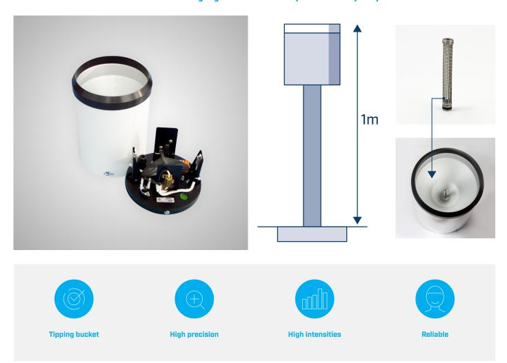
All rain gauges are made from non-corrosive materials. The funnel and also the circle in the upper part of the rain gauge, which creates the exact area for the falling precipitation (catching area of the rain gauge) - all these parts are made from aluminum alloy. The cylindrical casing is made from stainless steel.
