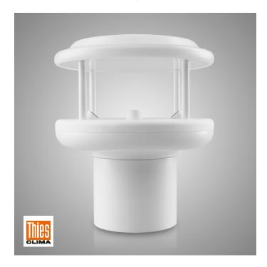
It measures wind velocity, wind direction, brightness, and precipitation. The wind velocity and wind direction are measured by an ultrasonic sensor in high-precision. The precipitation and its intensity are acquired via Doppler radar. A brightness sensor is included.
