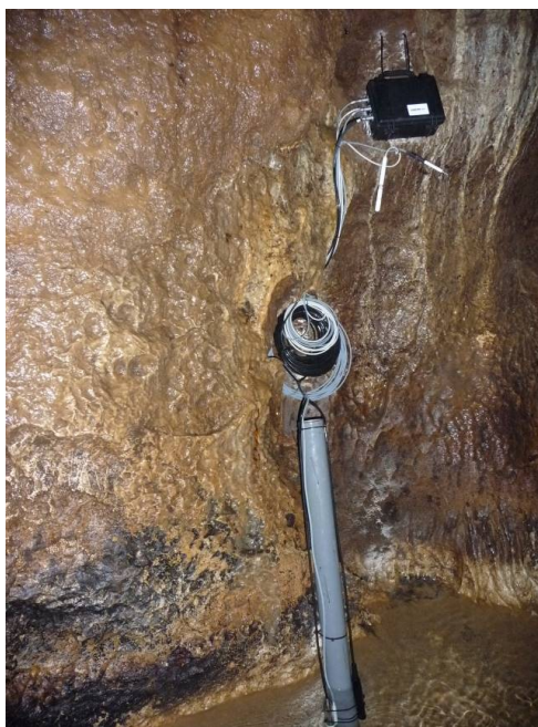
Mobile Monitoring Station with Air Temperature and Humidity Probes, Water Temperature, Water Level and Conductivity Probes and Data Logger
