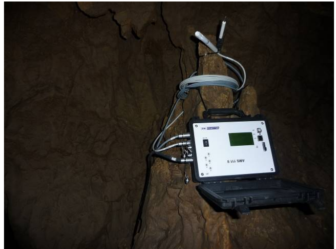
Mobile Monitoring Station with Temperature and Humidity Probes
